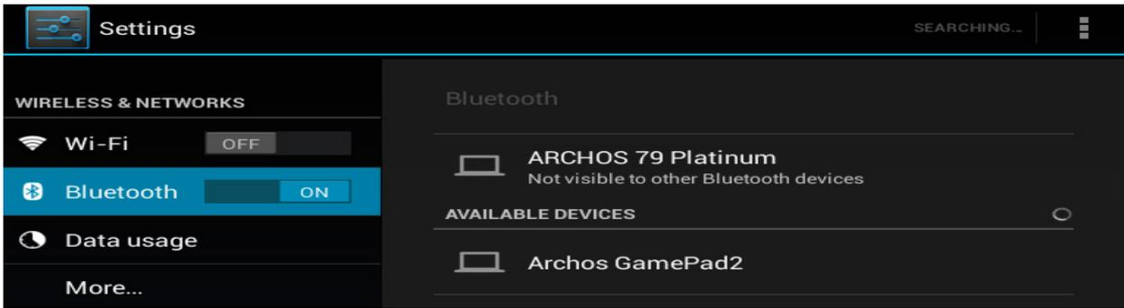
Press the name of the device you want to pair. A window will open with the name of the device and an automatically generated passkey. This window will also open on the device you want to connect. Press Pair on both devices.
