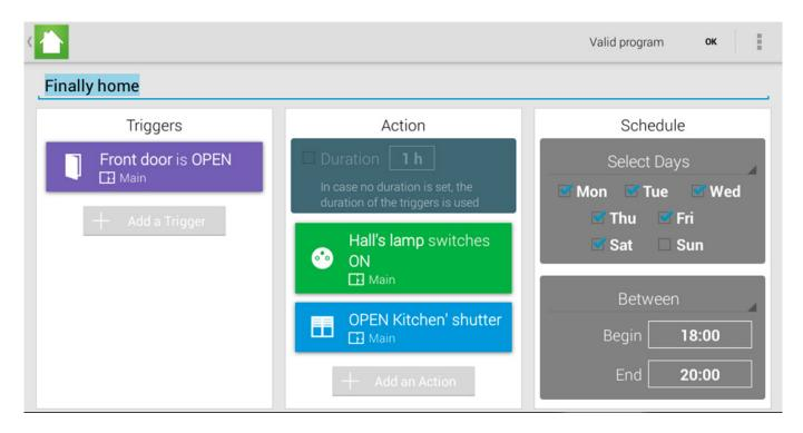
We set the Movement Tag on the opening of a door and choosed to switch on the plug on which the lamp is plugged as well as the opening of the shutters between 6 pm ro 8 om from Monday to Saturday.
